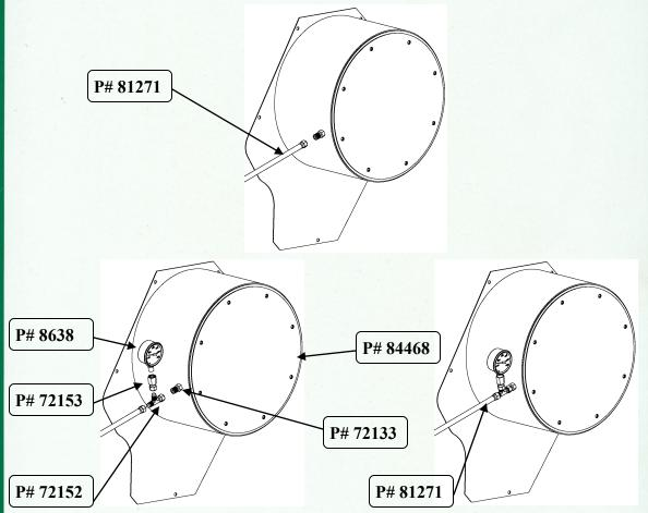
Connect T-fitting **P# 72152** to bulkhead fitting **P# 72133**. Connect JIC Female adapter **P# 72153**. Connect pressure gauge **P# 8638** to female adapter using Teflon thread tape. Reconnect hydraulic hose **P# 81271**. Tighten all connections.
